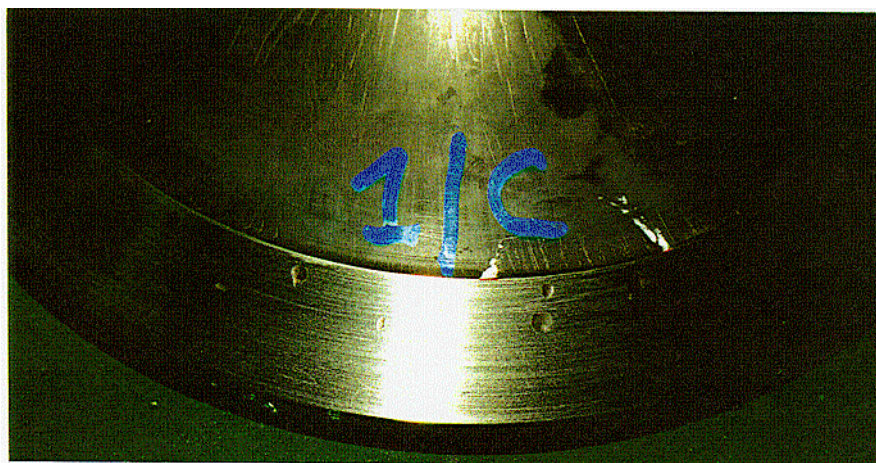
Photo 5: Acceptable seat condition after grinding
