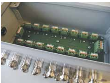
Fig. 10: Terminal box opened
