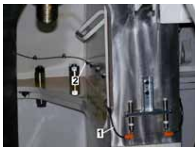
Fig.60: application of screwable cable holder in the engine
