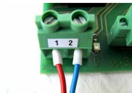
Fig. 74: Board power supply
