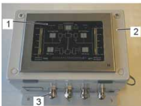
Fig. 79: Indication unit with cable glands
