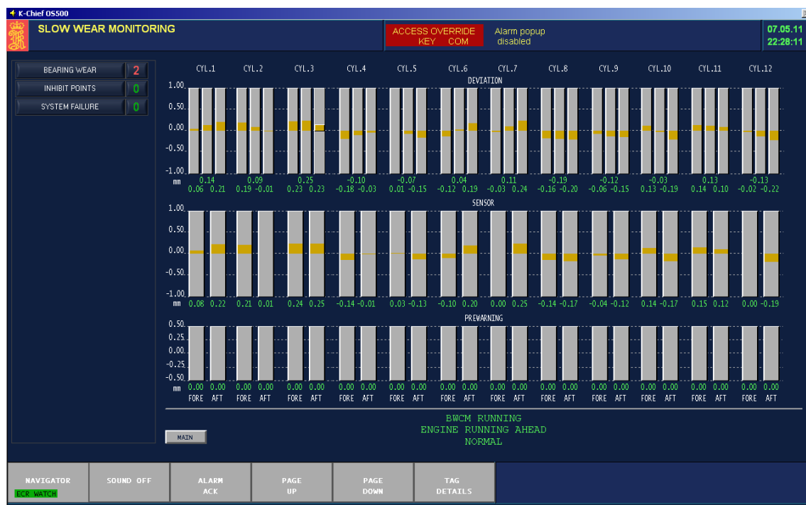
Figure 7 Bearing wear monitoring Slow Wear mimic
