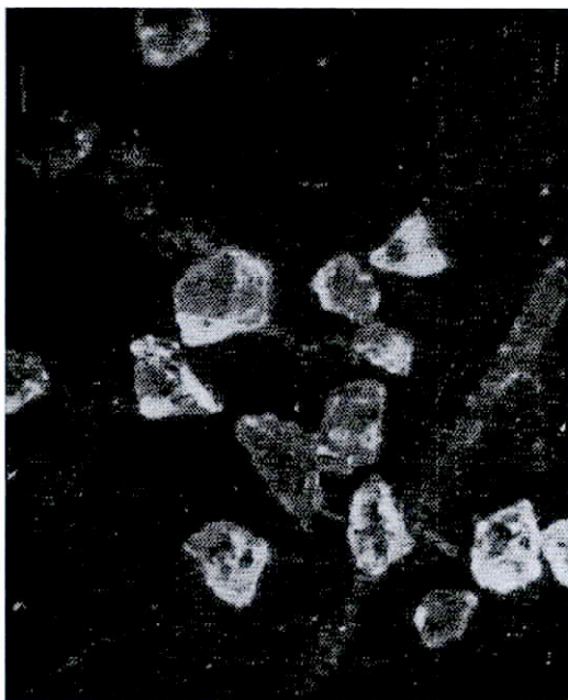
Photo 2 (X30) Hard particles (sand) separated from a sample of piston crown deposit . Oil and carbon have been removed by incineration, other matter by acid, magnetic separation and filtration. Theoretically these particles could have come into the combustion chamber either with the air or with the fuel.
