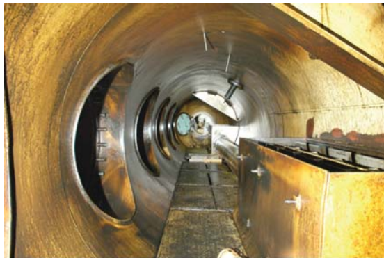
Scavenge Receiver, SLUDGE – S
