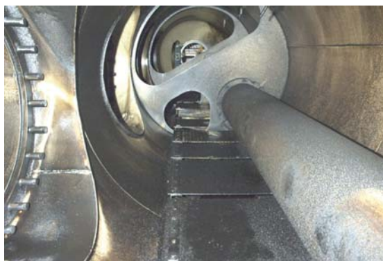
Scavenge Receiver, MUCH SLUDGE – MS
