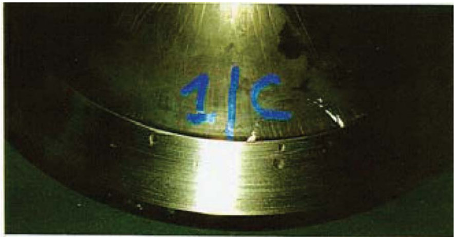
Photo 5: Acceptable seat condition after grinding
