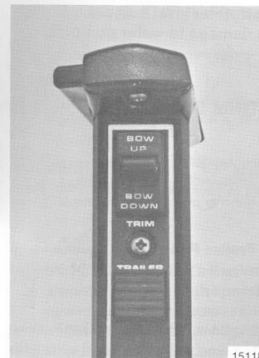
Figure 3. Power Trim Switches in Handle of Quicksilver Side Mount or Panel Mount Remote Control
