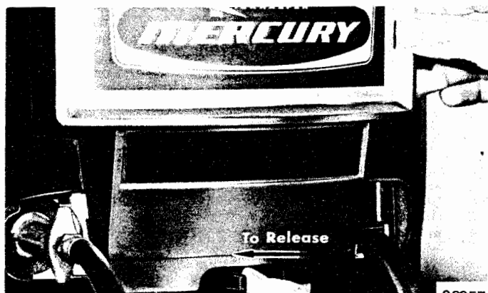
Figure 40. Removing Front Cowl - Merc 650 (3-Cyl.)
