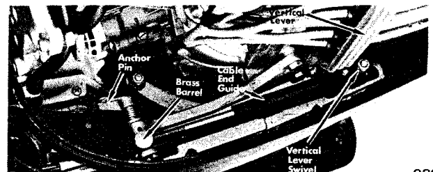
Figure 17. Throttle Cable Brass Barrel Secured with Anchor Pin
