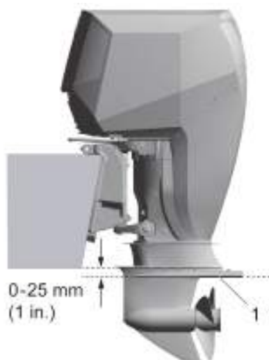
Fig. 9 Outboard mounting height
