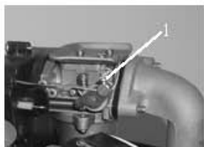
1. Throttle cable stop screw
