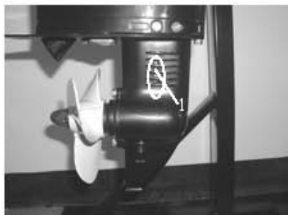
Cooling water passage inlet
