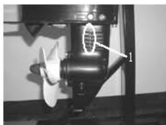
1. Cooling water inlet
