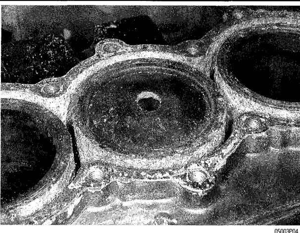
Fig. 15 A burned piston like this one will be replaced during an overhaul. The condition which caused the hole in the top of the piston must be identified and corrected or the same thing will happen again
