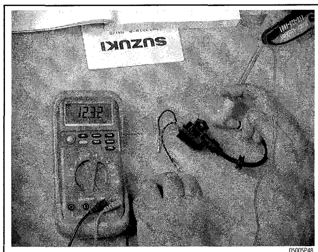
Fig. 23 The digital multimeter connection procedure for a continuity check will depend on how the coil is constructed
