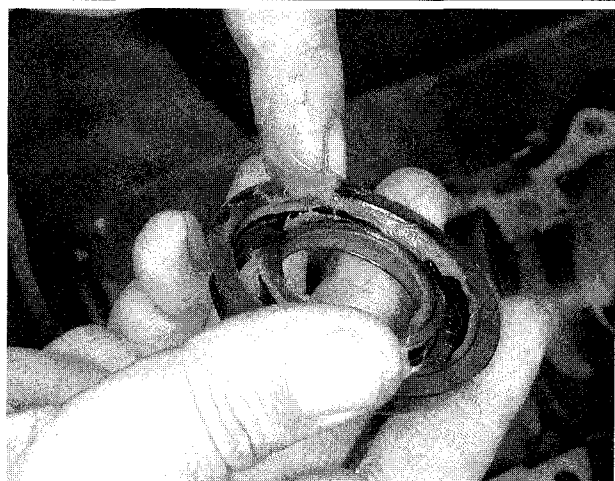
Fig. 62 Crankshaft seals should always be lubricated prior to installation
