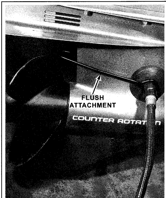
Fig. 85 This popular and inexpensive flushing device should be included in every boat owner's maintenance kit
