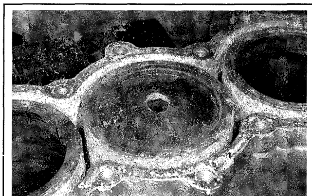
Fig. 6 A clogged fuel filter resulted in a lean fuel mixture at speed and caused the burn hole in the top of the piston. This powerhead required a complete overhaul
