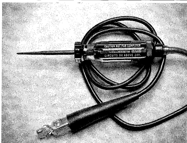
Fig. 8 A 12 volt test light is used to detect the presence of voltage in a circuit
