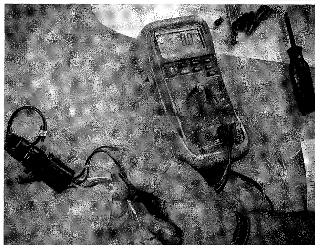
Fig. 11 Connect a multimeter between the switch harness leads and test for continuity
