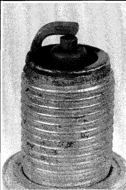
Fig. 39 A carbon-fouled plug, identified by soft, sooty black deposits, may indicate an improperly tuned vehicle. Check the air cleaner, ignition components and the engine control system.
