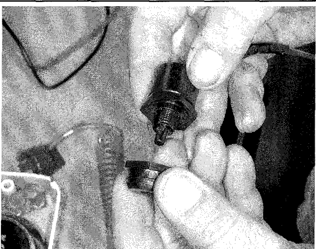
Fig. 9 The emergency switch is held in place on the remote control box by a locknut
