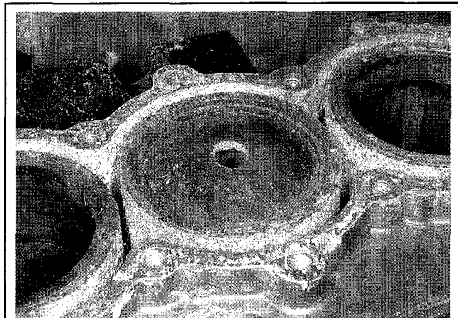
Fig. 25 This burned piston is typical of a combustion relate failure. The combustion chamber temperature got so hot that it melted the top of the piston (hole in the top of the piston)
