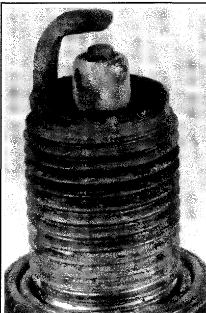
Fig. 42 This spark plug has been left in the engine too long, as evidenced by the extreme gap—Plugs with such an extreme gap can cause misfiring and stumbling accompanied by a noticeable lack of power
