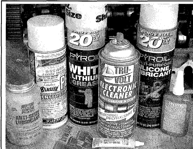
Fig. 13 Due to the very corrosive nature of salt water, some sort of anti-seize type thread compound should be used on all exposed fasteners outside of the cowling to reduce the chance of them seizing in place
