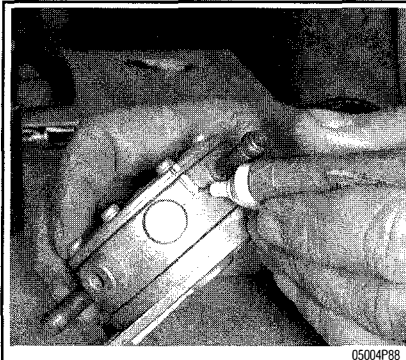
Fig. 17 When taking the pump apart, mark the pump sections for correct reassembly
