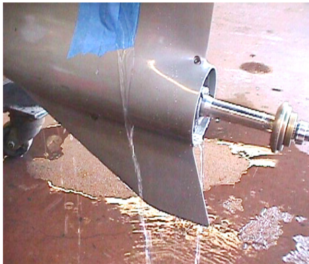
Figure 8 Drive Inlet Ports Taped Off (Duct or Shrink Wrap Tape)
