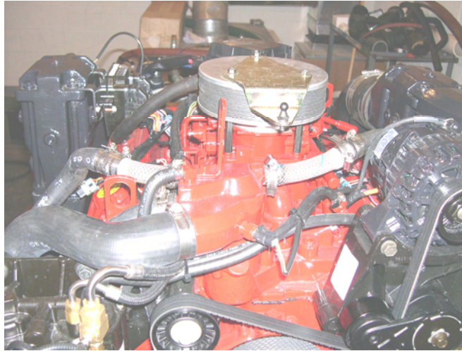
Figure 2 Clear Hose Setup on the Engine
