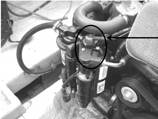
Fuel rail now has a pulse damper and NO regulator
