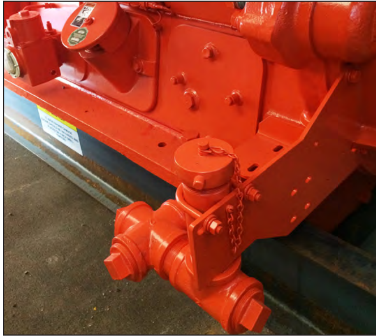
Figure 10-9: Oil fill location
