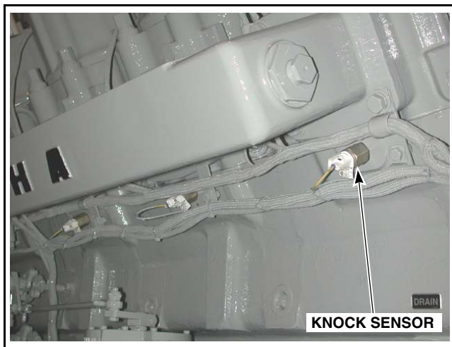
Figure 1.10-9 Knock Sensor (P/N A740110B)
