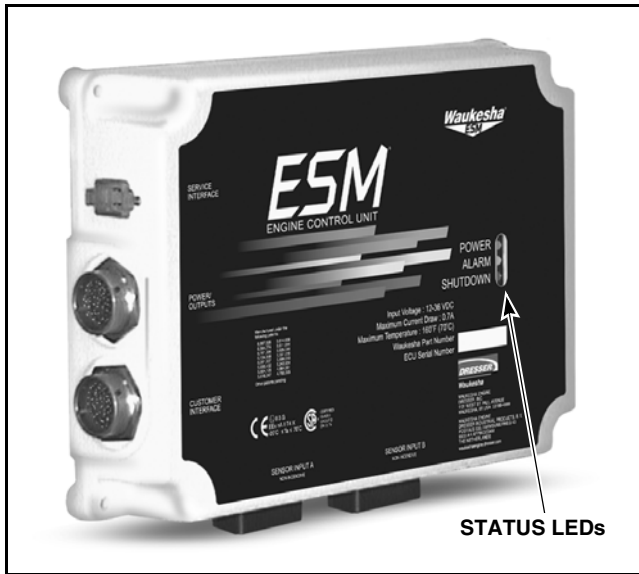
Figure 4.00-1 ECU Status LEDs
