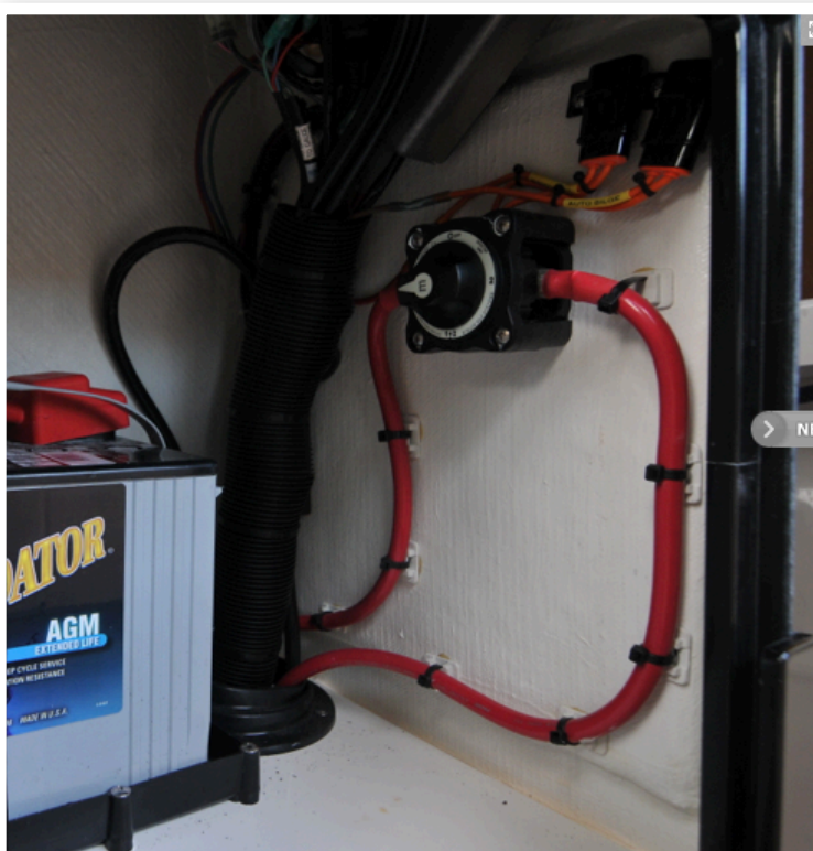
Battery Switch, Shown in Position 1
