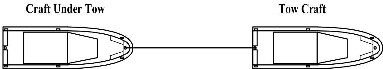
Figure 044-4.2a. Fore and Aft Tow
